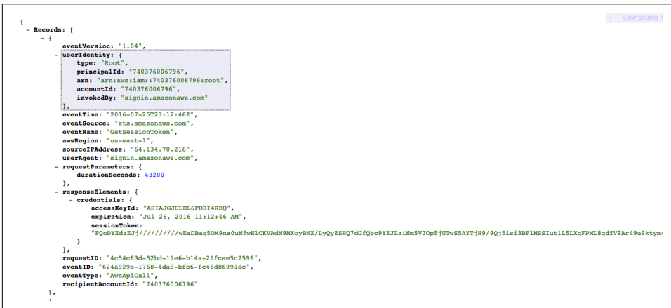
Figure 3-7. A CloudTrail login record examined inline in Chrome with JSONview—someone logged in as root, contrary to our policy!
