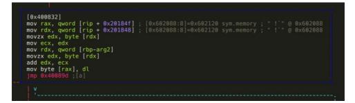
It basically loads an address from offset 0x602088 and adds *arg2* to the byte at that address. As r2 kindly shows us in a comment, 0x602088 initially holds the address of *sym.memory*, the area where we have to construct the "Such VM! MuCH reV3rse!" string. It is safe to assume that somehow we will be able to modify the value stored at 0x602088, so this "M" branch will be able to modify bytes other than the first. Based on this assumption, I'll flag 0x602088 as *sym.current\_memory\_ptr*:
