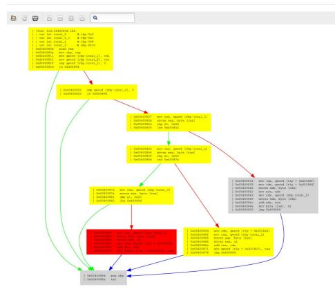
A sad truth reveals itself after a quick glance at these graphs: radiff2 is a liar! In theory, grey boxes should be identical, yellow ones should differ only at some offsets, and red ones should differ seriously. Well this is obviously not the case here - e.g. the larger grey boxes are clearly not identical. This is something I'm definitely going to take a deeper look at after I've finished this writeup.
