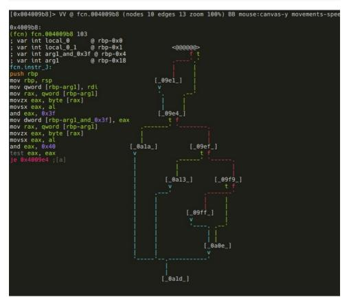
After the result of *arg1* & 0x3*f* is put into a local variable, *arg1* & 0x40 is checked against 0. If it isn't zero, *arg1\_and\_0x3f* is negated:
