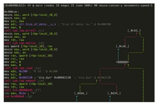
First, the "Size of data: " message we saw when we run the program is printed. So now we know that the local variable *local\_10\_6* is the size of the input data - so lets name it accordingly (remember, you can open the r2 shell from visual mode using the : key!):
