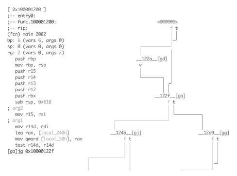
This mode allows you to see the disassembly of each node separately, just navigate between them using Tab key.
