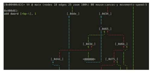
If the value is zero, the loop breaks and this block is executed before exiting:
