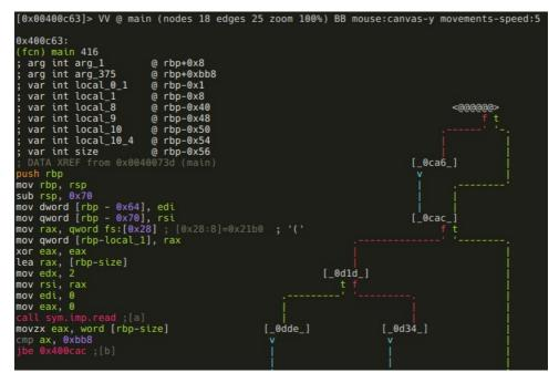
We can see that the program reads a word (2 bytes) into the local variable named *local\_10\_6*, and than compares it to 0xbb8. Thats 3000 in decimal, btw:
