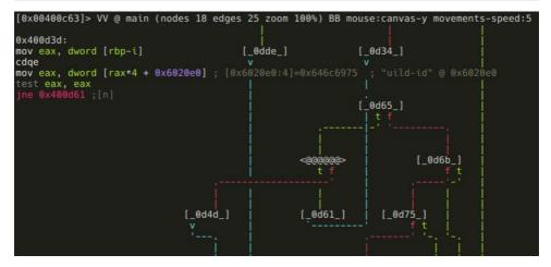
The memory area at 0x6020e0 is treated as an array of dwords (4 byte values), and checked if the ith value of it is zero. If it is not, the loop simply continues:
