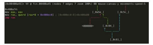
and r2 can't yet recognize jump tables (Issue 3201), so the analysis of this function is a bit incomplete. This means that we can't really use the graph view now, so either we just use visual mode, or fix those basic blocks. The entire function is just 542 bytes long, so we certainly could reverse it without the aid of the graph mode, but since this writeup aims to include as much r2 wisdom as possible, I'm going to show you how to define basic blocks.
