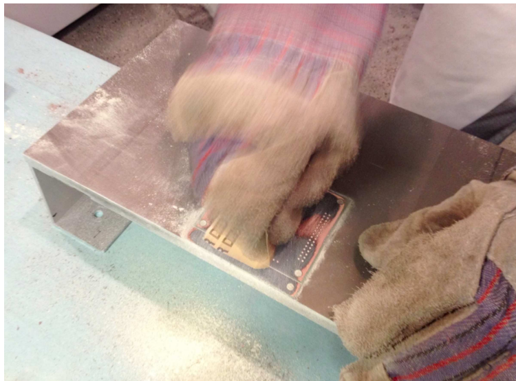
Figure 6.20: Sandpaper at work. You can see the copper of inner layer 2 starting to peek out from underneath the top substrate.
