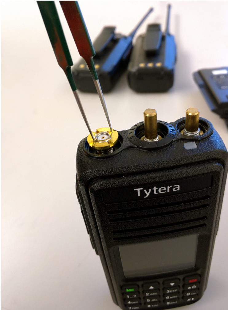
Figure 10.19: Removing the Antenna Rings
